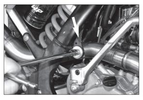
Caution: do not tighten the M8x20 screw included in the scope of supply until the exhaust system is completely mounted tension-free.
