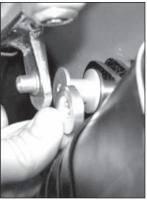
Use the M6x25 with DIN125 A6.4 washer for the front clamp. Use the M6x50 with DIN125 A6.4 washer for the rear clamp.
