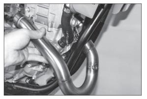
Mount the shock absorber, mount the Akrapovic header pipes, align and fasten with the exhaust springs included in the scope of supply.
